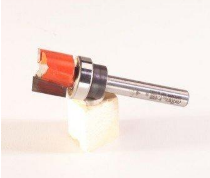
Photo 3 – Use a 5/8-in. diameter, 1/2-in cut length pattern bit with the jig. A pattern-cutting bit features a guide bearing that is located above the cutter head.
