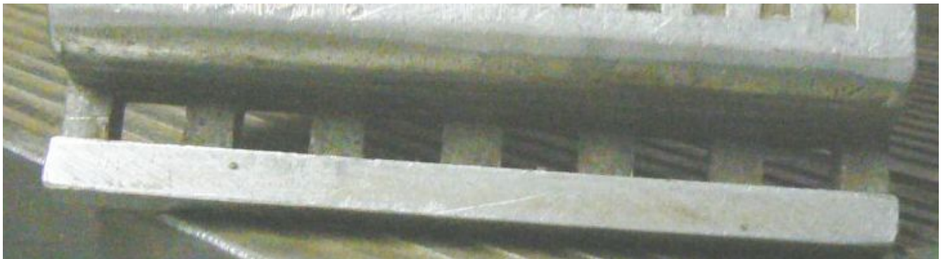
Extension table front showing cast in fence reference(under side beveled)
