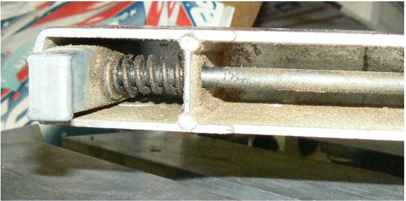
Mark 5 rip fence rear clamp bottom
