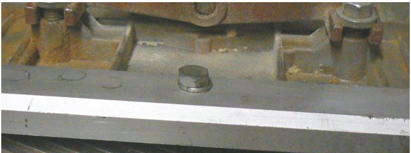
Mark 5 main table front extrusion – Used by fence as a position reference
