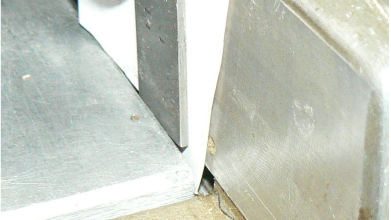
Fence to slot bar and paper shim
