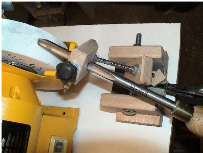
The finished Jig with gouge fitted for trial run.
