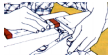
Fig. 2: Wrap an oilstone in waxed paper, leaving one end exposed. Place it on the infeed table so that the exposed part of the stone rests on the bevel of one of the knives.
