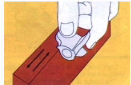
Fig. 8: Use the edge of a stone to hone the entire face of Shaper Cutters.
