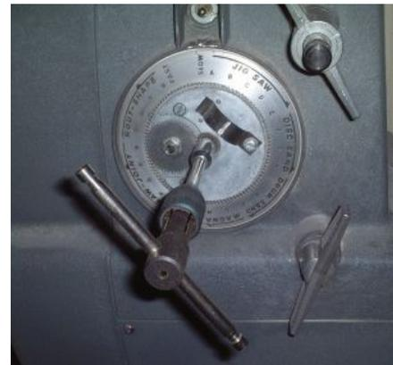
Turn off your Shopsmith. Re-tighten the jam nut. Press in and turn the speed dial until it reads "fast."
