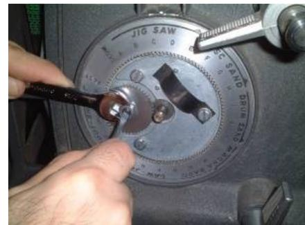
If the high speed stop engaged before the drive belt was near the edge of the motor pulley, turn the set screw COUNTERCLOCKWISE and, at the same time, turn the worm shaft CLOCKWISE until the belt is between  $\frac{1}{8}$ " and  $\frac{1}{16}$ " from the outer edge of the pulley. Note the use of pads on the pliers-this is to protect the worm shaft. This is the Shopsmith recommended procedure.
