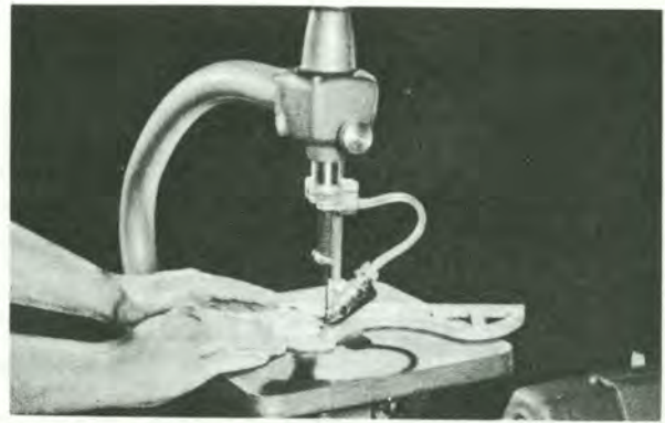
Fig. 9 Drill hole for each section
