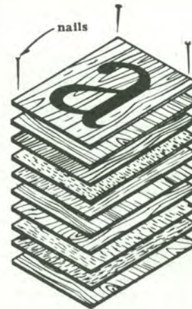
Fig. 10 Use one pattern to cut duplicate pieces
