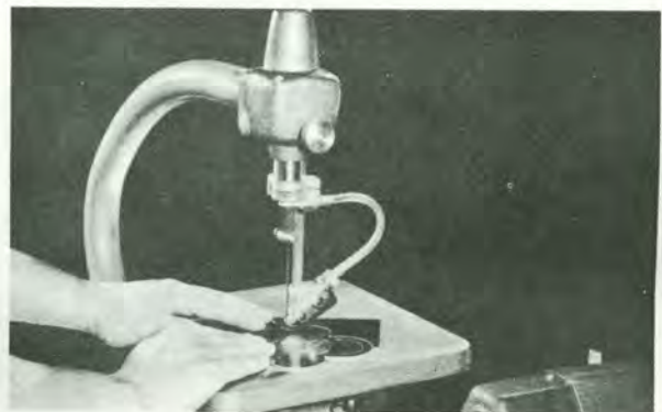
Fig. 12 Metal cutting is another Jigsaw operation
