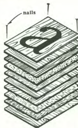
Fig. 10 Use one pattern to cut duplicate pieces
