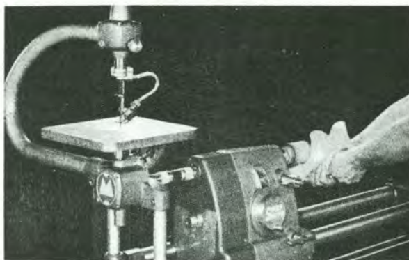
Fig. 14 Jigsaw-Drum Sander combination
