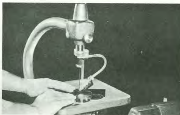
Fig. 12 Metal cutting is another Jigsaw operation
