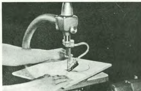
Fig. 8 Feed slowly, do not force blade
