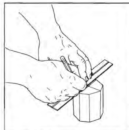
Figure 4. To find the center of a workpiece, draw two intersecting diagonal lines corner to corner on each end of the workpiece.
