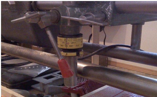
Using feeler gage on non-adjustable collar
