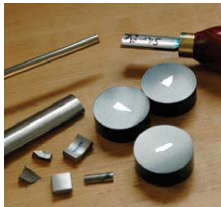
Sections of lathe tools embedded in composite materials and prepared for emission (spark) test.
