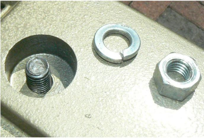
Pretty obvious, but the lock washer goes on first followed by the nut. At this time only finger tighten the two nuts.
