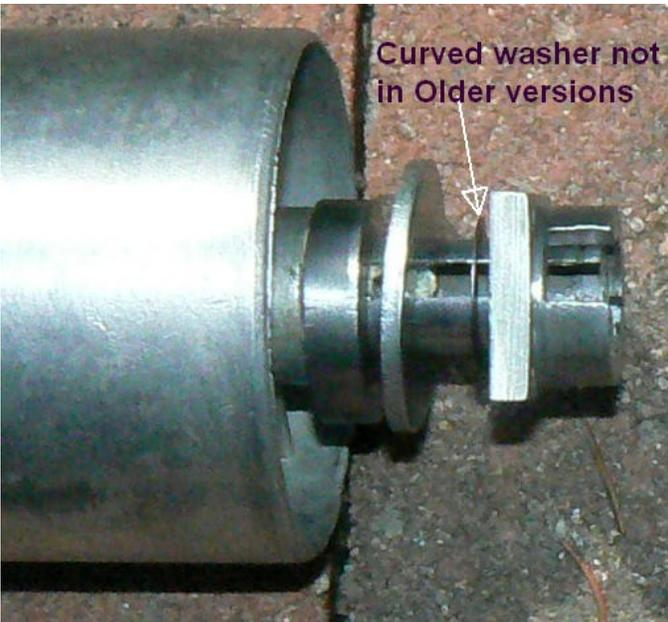
The 'knob' end of the idler drum has two or three parts to put back on. The large flat washer goes on first. Then on newer versions, a curved washer followed finally by the 'guide bushing'. The idler drum was cleaned out of old original grease and replaced with lithium grease. Not easy to do, but the ends will pull out(under spring tension) and provide access to the grease and each end of the shaft where the bearing bushings contact the shaft. Need extra hands or vise to do that.!
