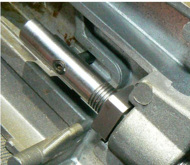
As promised a pix showing the fixed tracking screw roll pin properly inserted with the roll pin facing out into its groove.
