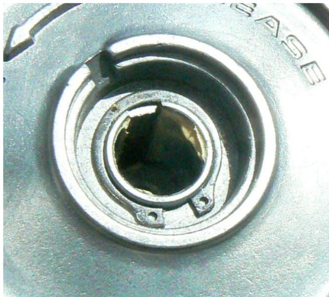
I think it a good idea to position the open end of the ring away from the open slot on the shaft.
