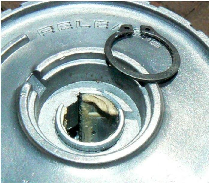
The knob is retained onto the shaft by an external ring that fits into a shallow groove near the end of the shaft.
