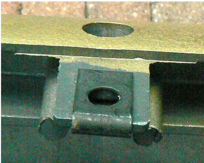
The older version has platen mounting tabs that are below the edge of the casting which requires the use of 2 thick spacing washers under each of the six platen mounting screws.
