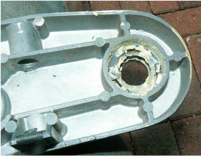
A word about the bearing cavities in the side castings. There is a spring clip in the bottom that is **installed with the fingers facing the bearing (flat side to the bottom)**. That white stuff is lithium grease (both sides of the clip). It has been pointed out that SS CS says the reverse when asked. So flat side s/b against the bearing, and the fingers towards the bottom of the hole. Mine were the other way when I disassembled it???
