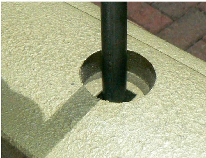
If the bolt is held vertical over the square hole in the casting and the assembly is positioned correctly, the bolt will drop straight down into the hole on the opposite casting.
