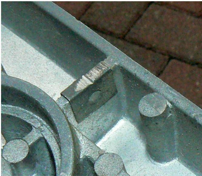
On the back side of both castings there are two clips on each that serve as sacrificial lambs when the belt tracks too close to either side. The hardened tinnerman clips will last longer than the softer aluminum casting.
