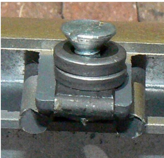
This pix is of a newer version and shows the platen mounting tabs are raised above the side of the casting. This eliminates the need for the 12 spacer washers (shown below) used in this older version. Yes the rust indicates it resides in the 'to do' pile.
