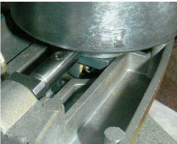
Finally the idler drum etc. installed in the casting. Notice the tracking screw is inside of the large flat washer so as to properly contact the tension cam. The guide bushing is riding in its slot and the tension pin is in its groove.
