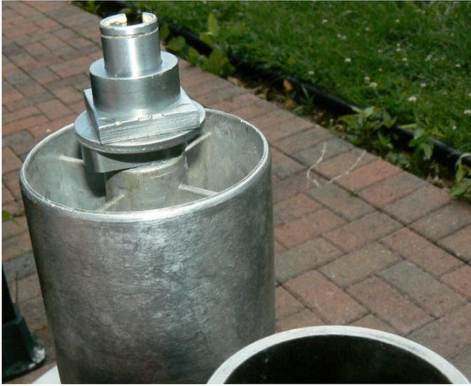
Insert both spacers in their bores and position the guide bushing so that the long sides run front to rear(so it will fit into the slot in the second casting).
