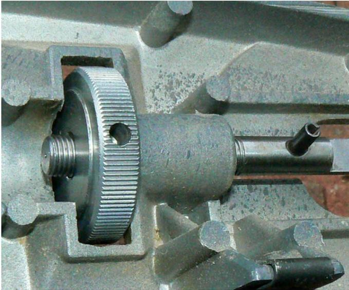
The tracking adjustment knob and screw is inserted in the hole and pre-adjusted to about 1/2" thread sticking out the rear(that includes the knob thickness). More about that 1/2" later! See post #5. This is not critical since it can easily be adjusted even with a belt installed. Note the side of the tracking adjustment knob with the raised center faces towards the center.
