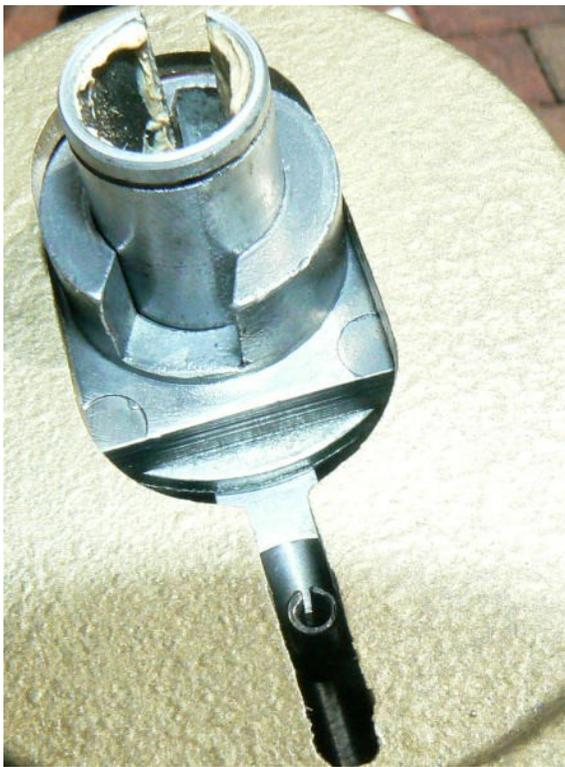
After sliding the casting onto the drive drum shaft and the two spacers and the guide bushing, the idler shaft etc. should look like this.(Yes all that at once is a bit of a challenge, but perseverance will get it done) Notice the tracking screw roll pin, the tracking screw end and the guide bushing are all in the proper place.(Just like the other side).
