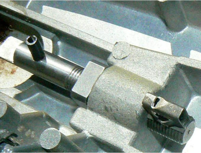
The other side has a fixed(but still adjustable with the belt off) tracking screw and it also should be installed with 1/2" exposed threads towards the rear. The tinnerman clip removed is 1/2" wide so it is a good gauge. More about that 1/2" later See post #5
