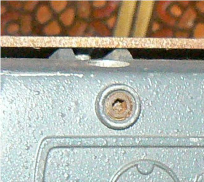
This pix is of a newer version and shows the platen mounting tabs are raised above the side of the casting. This eliminates the need for the 12 spacer washers (shown below) used in this older version. Yes the rust indicates it resides in the 'to do' pile.
