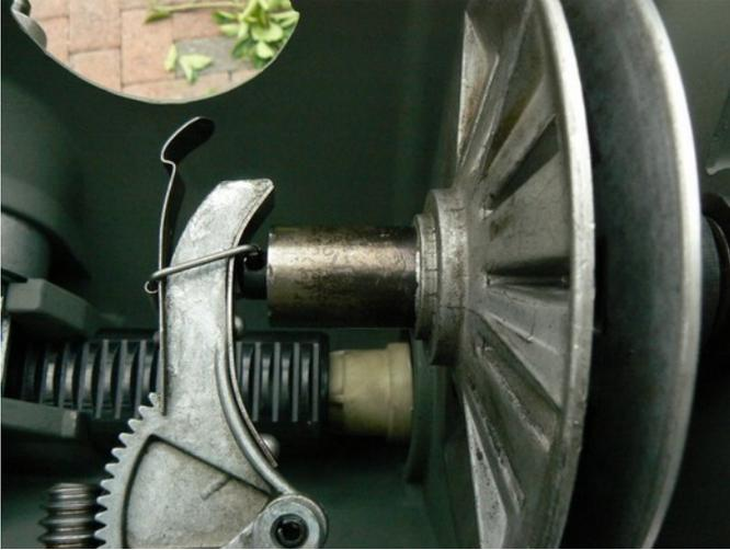
With the speed control set to the high speed stop position, from the inside of the headstock, slip the square shaped 'ring' over the quadrant arm. Depress the flat spring (with a step near the end) to get the loop onto the arm. NOTE: This pix was taken with the speed control set to slow. The square 'ring' slips over the quadrant arm when set to high speed.
