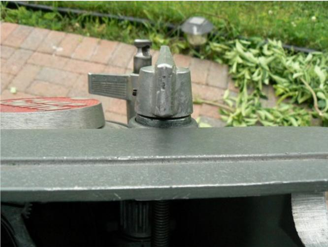
Adjust the wedge on the end with the wingnut so it is all the way towards the wingnut.
