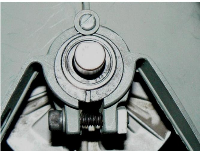
If there was a screw/washer at the top of the idler shaft bore replace it and tighten. Snug the bolt securing the eccentric bushing. If adjusting the drive belt tension now, rotate the eccentric bushing until slight pressure deflects the drive belt about 1/4". This pix shows the eccentric bushing before tensioning drive belt.
