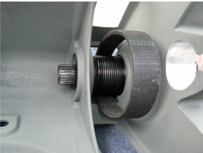
This pix shows the shaft **ALMOST** all the way in with the drive belt around the pulley.
