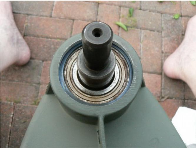
This shows the retaining spring completely installed. Make sure the entire spring seats into the groove.
