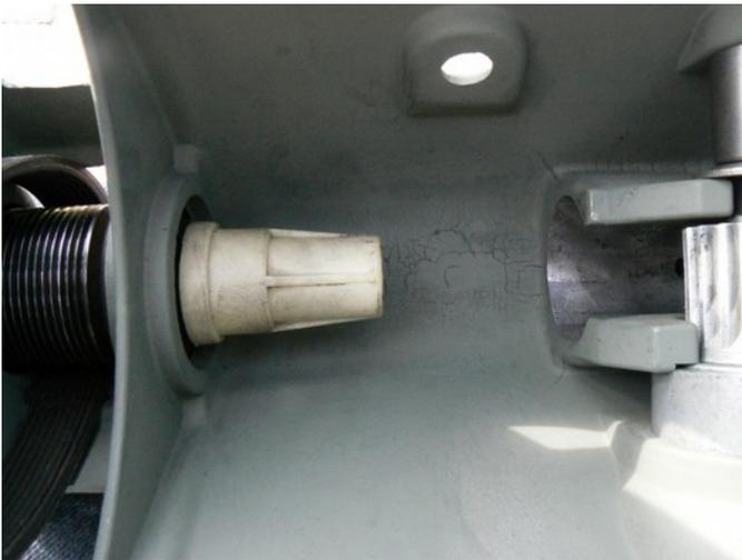
Slip the nylon quill shaft/upper shaft coupler onto the upper shaft. Start the coupler onto the upper shaft by aligning the splines with the coupler. Apply sufficient further force to expand a spring inside the coupler which will cause the coupler to 'snap into place' in a groove in the upper shaft.
