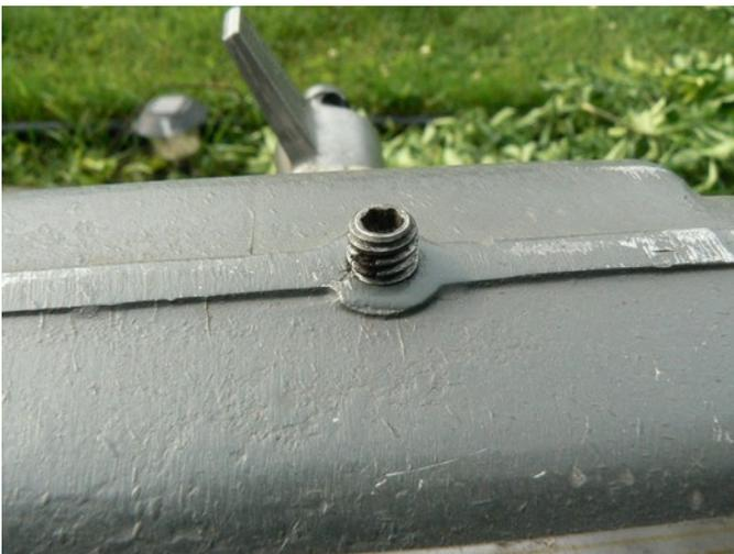
Carefully drive the setscrew until it bottoms out into the **BOTTOM** of the keyway. Back the set screw out about 1/8 turn. Advance and retract the quill to verify the screw **DOES** limit the quill travel, but does **NOT** drag against the bottom of the keyway. Adjust the setscrew if needed. Notice the setscrew has a nylon insert plugged into the threads. This serves as a method to keep the setscrew from moving(it is not tightened).
