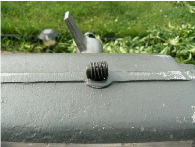
Notice the projected end on the setscrew. This end **MUST** go into the keyway on the top of the quill. When inserting the setscrew, be careful so as to **NOT** drive the setscrew into the side/edge of the keyway.
