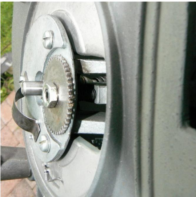
Adjust the speed control all the way to the high speed stop. This is determined by the quadrant arm stopping against the stop screw. Notice the small spring located near the top(lower left in pix). Do not forget to install it before putting outer ring in place. The end with a sharp bend goes into a hole on the right and the straighter end slides in a groove on the left.
