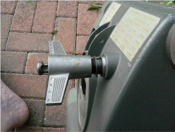
Slip the spring washer and wing nut onto the 'other' end of the quill feed shaft and lightly snug it up.
