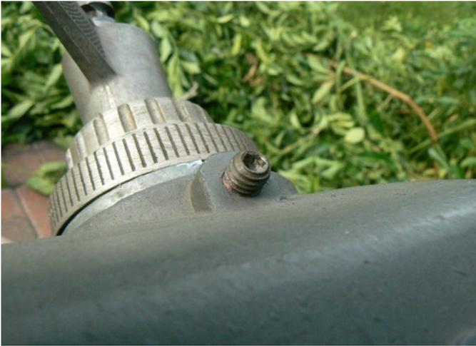
Sight down into the setscrew hole and align spring housing with previous marks left by the setscrew. You may need to loosen the wingnuts to orientate the housing etc.
