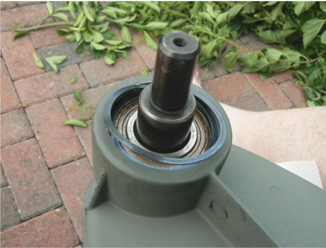
Make sure the shaft and bearings are seated all the way into the headstock. The back edge of the rear bearing should just clear the front edge of a groove at the back of the bore. Start the retaining spring into this groove. Start with the end and rotate it around while applying pressure so the end inserted does not come out.
