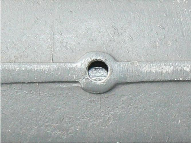
It does not show too well in this pix, but the keyway on the top of the quill needs to be centered under this setscrew hole.
