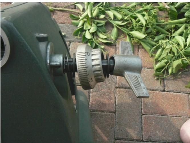
Note the positioning of the quill spring housing is incorrect. The index mark should point towards the set screw.
