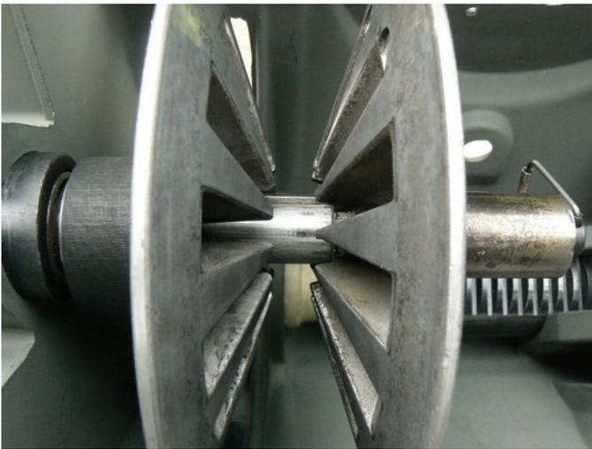
Slide the Control sheave onto the idler shaft. The shaft has a key and the sheave has a keyway slot which must be aligned. This would be a good time to lubricate the control sheave/shaft. Finally slip the Motor belt over the control sheave/shaft.
