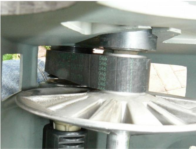
Notice the groove in the center of the bearing. This groove allows the set screw which has a cone shaped end to position the bearing in the eccentric sleeve and secure it. DO NOT overtighten this setscrew as it might apply too much pressure on to the bearing.
