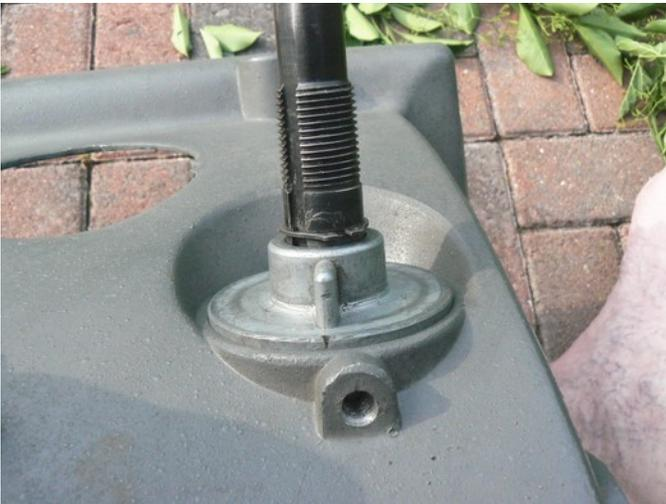
Notice the index mark and feed stop are at the 'top' of the 'larger' hole. Slip the retaining ring onto the shaft and into the groove.
