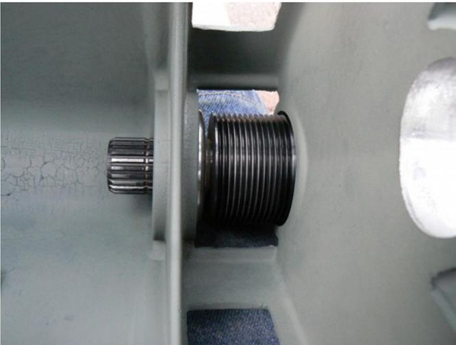
Continue pushing the drive shaft and bearings into the front bore. **RESIST** the temptation to **FORCE** it. Gentle tapping should be all that is required. If it gets 'stuck', back it out and start over.
