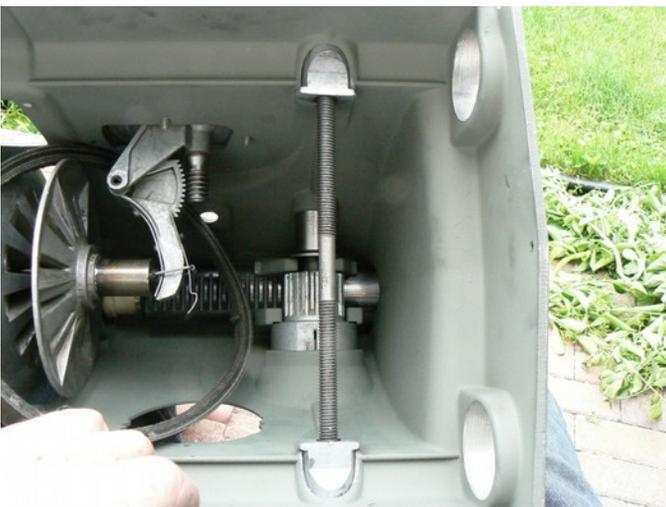
Position the wedge on the wingnut end against the inside of the headstock casting. Adjust the wedge on the OTHER end so as to also be against the inside of the headstock casting on the opposite side. Rotate both wedges so as to position the flat clamping surface away from the top of the headstock(the pix is from the bottom looking up). Snug the wingnut so as to position the wedges for later insertion of the headstock onto the way tubes.
