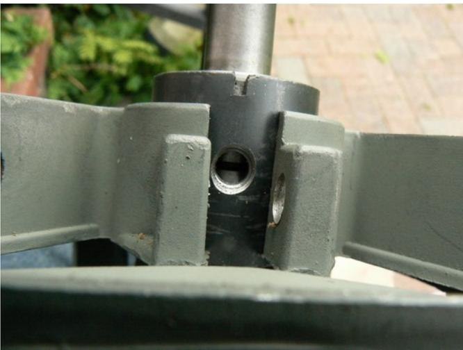
Position the bearing eccentric bushing onto the idler shaft bearing with the adjusting slot facing the end AWAY from the pulley. From the INSIDE of the headstock Slip the Drive belt(poly-v/Gilmer) onto the grooved/cogged pulley. For THIS vintage Poly-V belt the belt should be positioned so as to just cover the third GROOVE of the pulley on the drive shaft(upper)(there should be two GROOVES showing on the end of the drive pulley facing the quill handle etc.).
