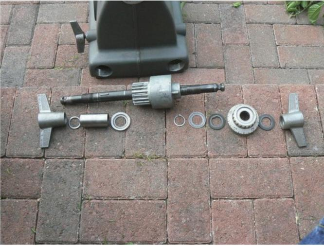
This shows the sequence the various parts are assembled onto the quill feed shaft. **Early Mark 5 did not have the flat washer between the retaining ring and the first serrated washer.**[3/21/2012]
