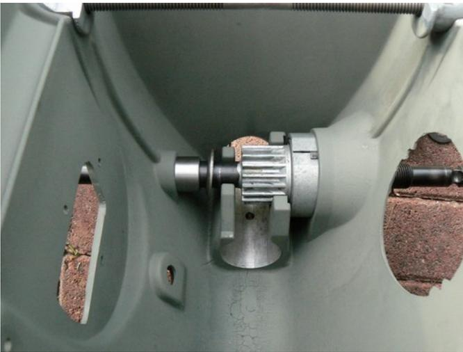
Slide the quill feed shaft into the headstock. The spring housing goes into the larger headstock hole. Slip the cup washer and sleeve on to the shaft at the other end. Notice the orientation of the cup washer. The 'flat' outer circumference faces the casting 'ears'.(faces right in the pix) The sleeve has a keyway in the inside which must align with a key on the shaft.
