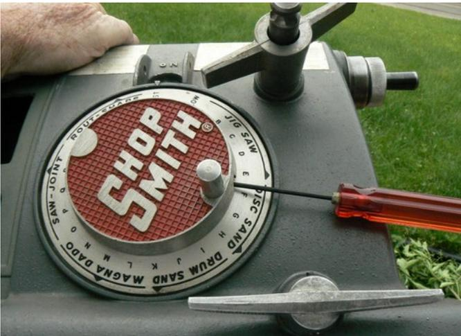
Position the outer ring to indicate 'fast'. Notice the shaft on to which the knob attaches has a 'dimple' drilled into it. The knob set screw MUST be tightened into that depression. Slide the knob onto the shaft and feel the screw centering into the 'dimple' by rocking the knob back and forth. Tighten the set screw at the center/bottom of the 'dimple'.
