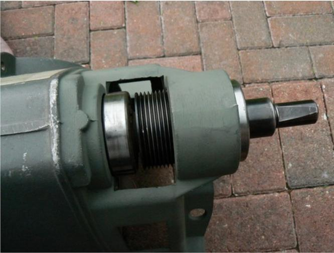
Slide the drive shaft front bearing with the splined shaft first **THROUGH** the rear bore. The drive belt should be positioned so that the front bearing passes through the belt.
