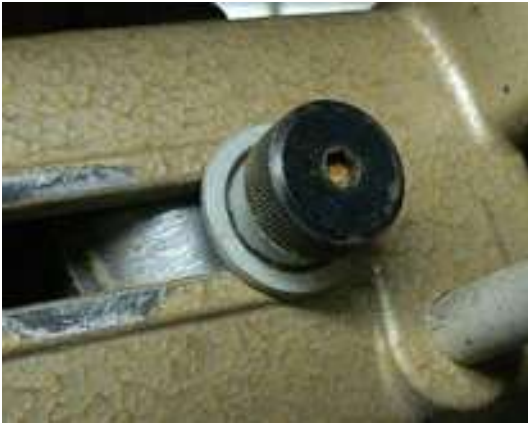
The 3/8-16 mounting screw with 5/32" hex socket.
