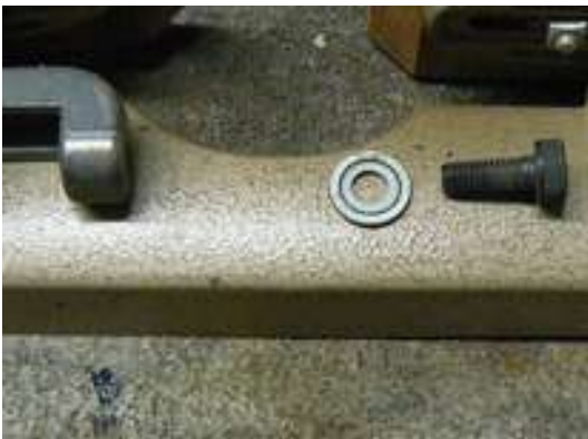
The Mark 5 mounting screw, washer and under table clamp(a pair fits over the front and rear edges of the work table).
