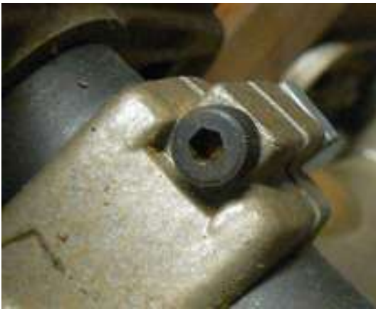
The 1/4-20 screw with 5/32" hex socket.
