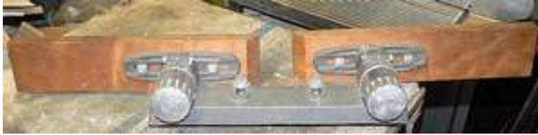
Before breakdown. Notice the location of the mounting screws.
