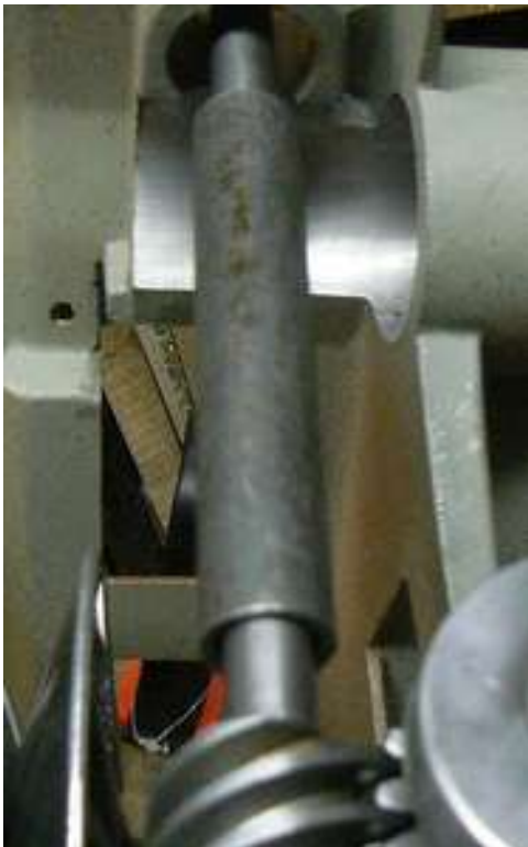
Next on the shaft is a long spacer.
