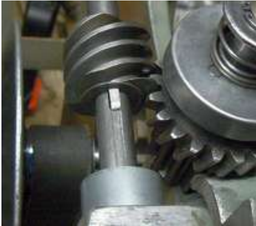
The worm gear is slipped onto the shaft. A small woodruff key goes into a keyway in the bore of the gear. The worm gear meshes with the bevel gear on the counter shaft.
