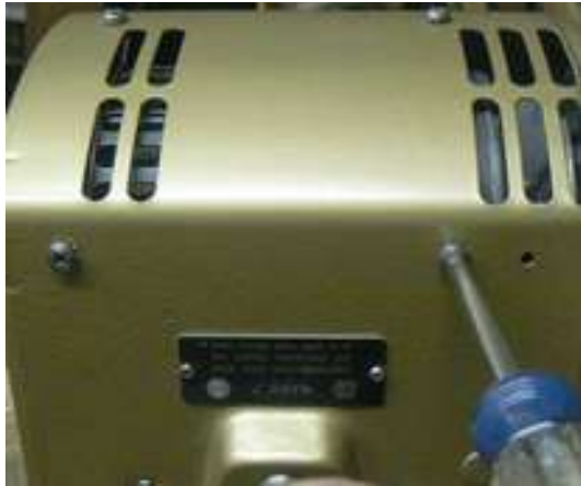
At last we mount the motor. The Mark VII differs from the Mark 5/V as the mounting brackets use 2 of the 4 screws on the front. The screws are still #3 Phillips.
