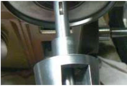
The spacer is inserted into the crank hub.
