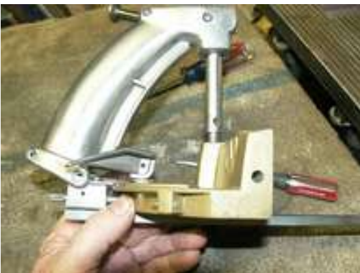
Not shown in the pix, is the mounting post which fits into the area under the pivot plate screw. The relief cut into the post sets on the narrow area of the 'hole'. The other half of the handle is placed onto the pin punch and meshed with the first half. By inserting the screw as the assembly is drawn off the pin punch keeps the pivot plate from shifting out of position. The top two screws are tightened.
