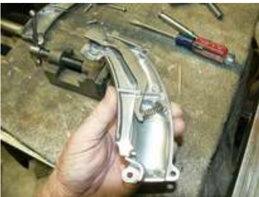
So is this, but assembly can be trying! Using a table vise and drift pin punch makes it easier. Notice how the parts nest. Squeeze handle in the groove, pivot plate in the notch and spring on the nubbin of the pivot plate and spring in the 'box'.
