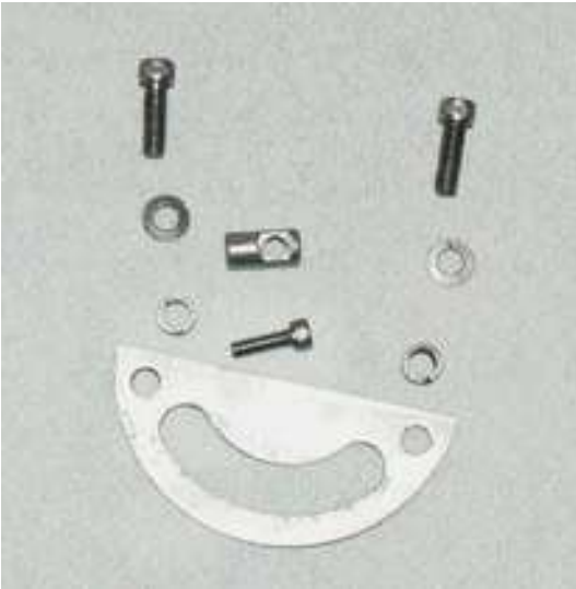
After evaporust wire brushing and JPW(original)
