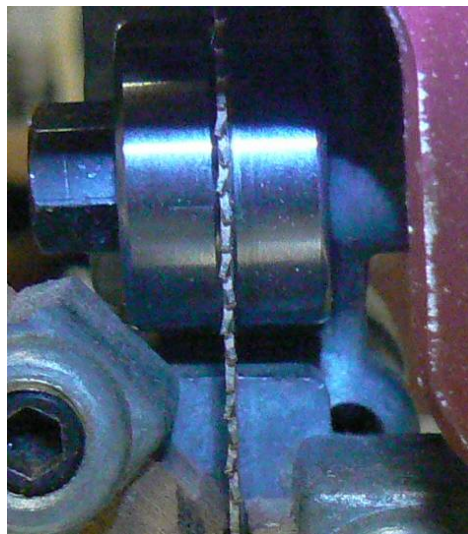
Lower Position Blade Centered And Clearance
