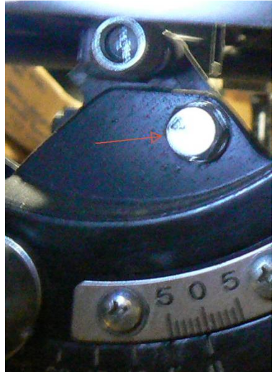
Lower Bearing Bracket Slots
