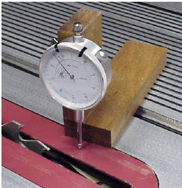
The jig holds the dial indicator vertical to the surface. This can be used to shim table inserts to be flat with the table, adjust depth of cut of dado blades, and even adjust the depth of router bits.
