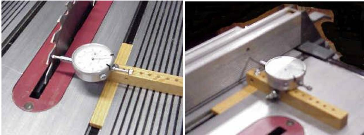
Alignment jig made of hardwood and an inexpensive dial indicator. The above jig, consists of a rail that fits snugly in the miter slot and is bolted to a .75" square piece with holes drilled so the rail can be mounted at many positions and the dial indicator mounted at two positions
