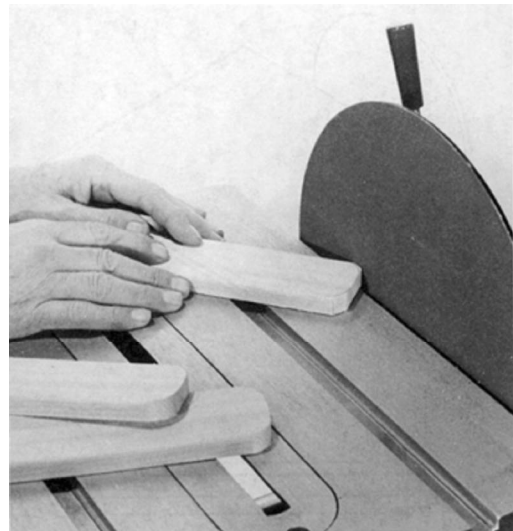
Figure 27. Corners can be rounded off by sanding to a line. The bulk of the waste should be removed with saw cuts before you begin.
