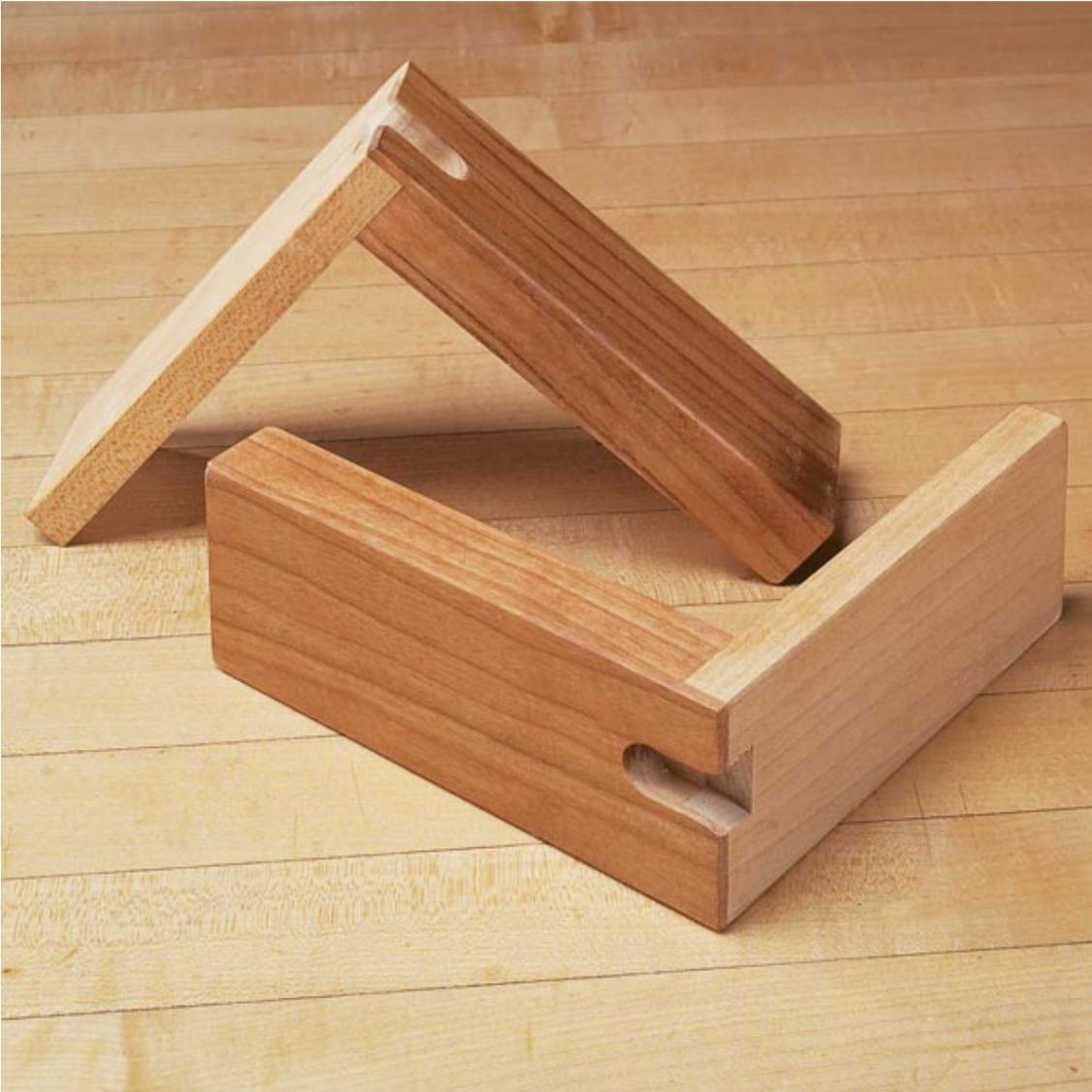
Make clamping blocks. An L-shaped clamping block the same thickness as your workpiece keeps the clamping bar from "racking" so they'll apply consistent pressure across the workpiece. Then, once you have a perfect cut, rout a dovetail in the block to use as a depth gauge for your next project.
