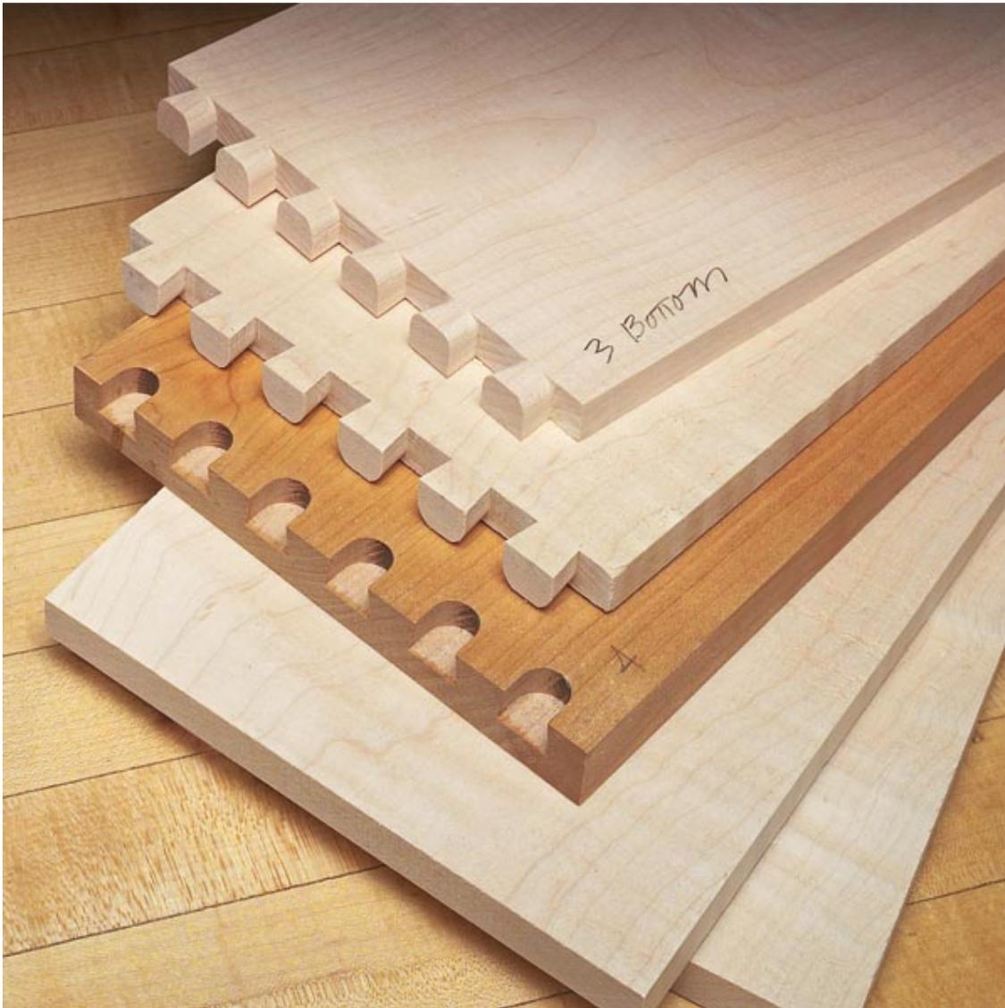
It might take some trial and error to get the exact setup for a perfect joint. Have plenty of extra stock on hand for test cuts. And be sure to use stock milled to the same thickness that you'll be using to construct your drawers.
