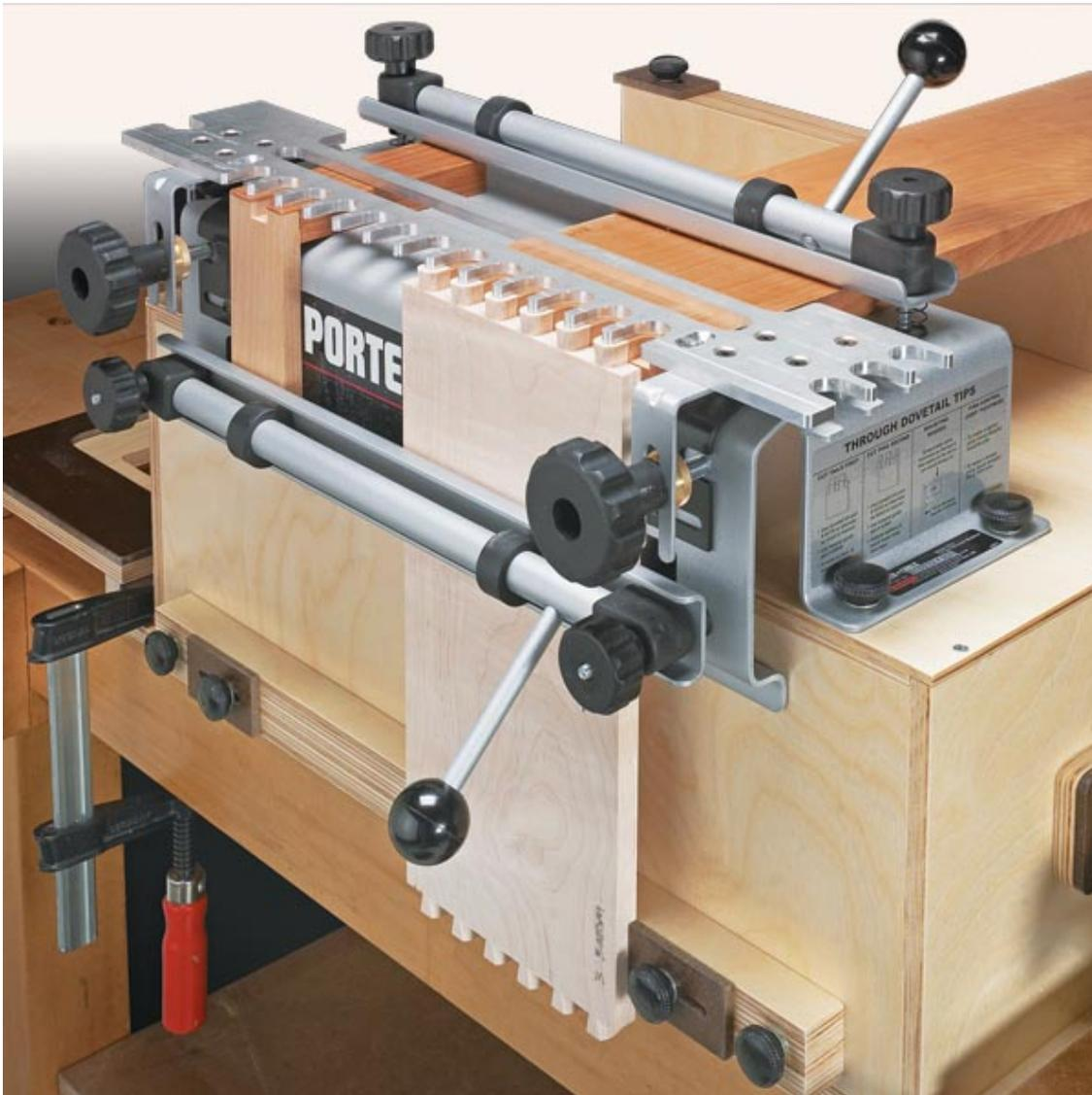
Chipout sometimes occurs on drawer sides. One trick that can eliminate chipout is making a light scoring cut along the front of the drawer side before cutting the dovetails. You can also start with wider workpieces and then trim them to size, removing any tearout that may occur at the edges.
