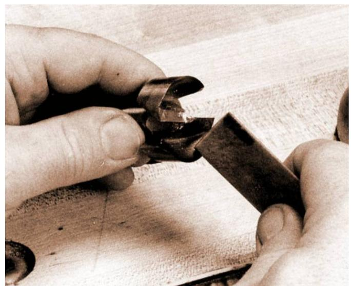
This guide holds both spade bits and brad-point bits, helping guide the file as you sharpen. When sharpening spade bits, use the angled end of the jaw that's cut 10 degrees off square. For brad-point bits, use the jaw that's 20 degrees off square.
