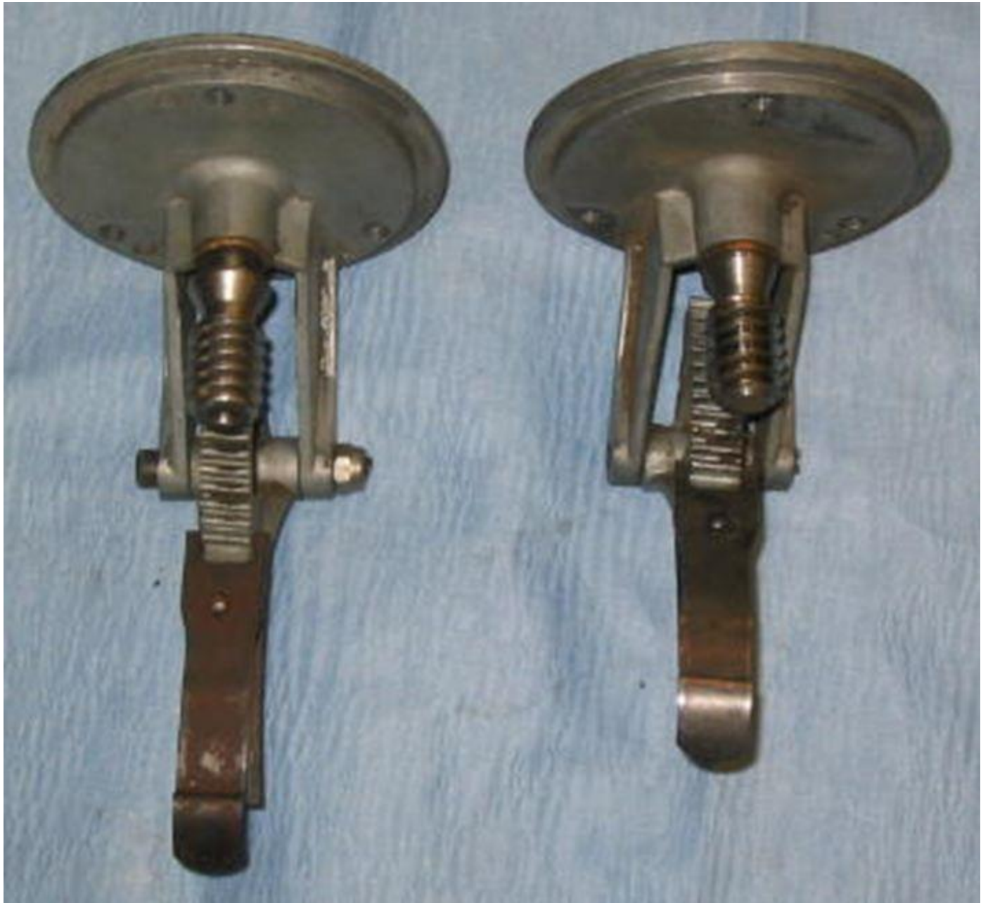
This picture shows the removed Speed Control Assembly on the right side and a rebuilt Speed Control Assembly on the left side.
