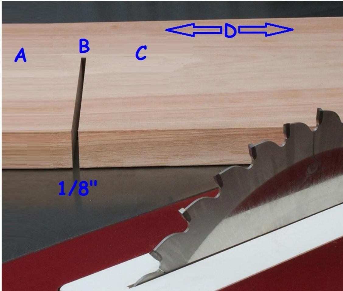
As illustrated above, the blade cut a 1/8" kerf out of board A, theoretically leaving;  $A^* = 12"$   $B = 1/8"$  and  $C = 5 \frac{7}{8}"$  accounting for all 18" of the original material in A
