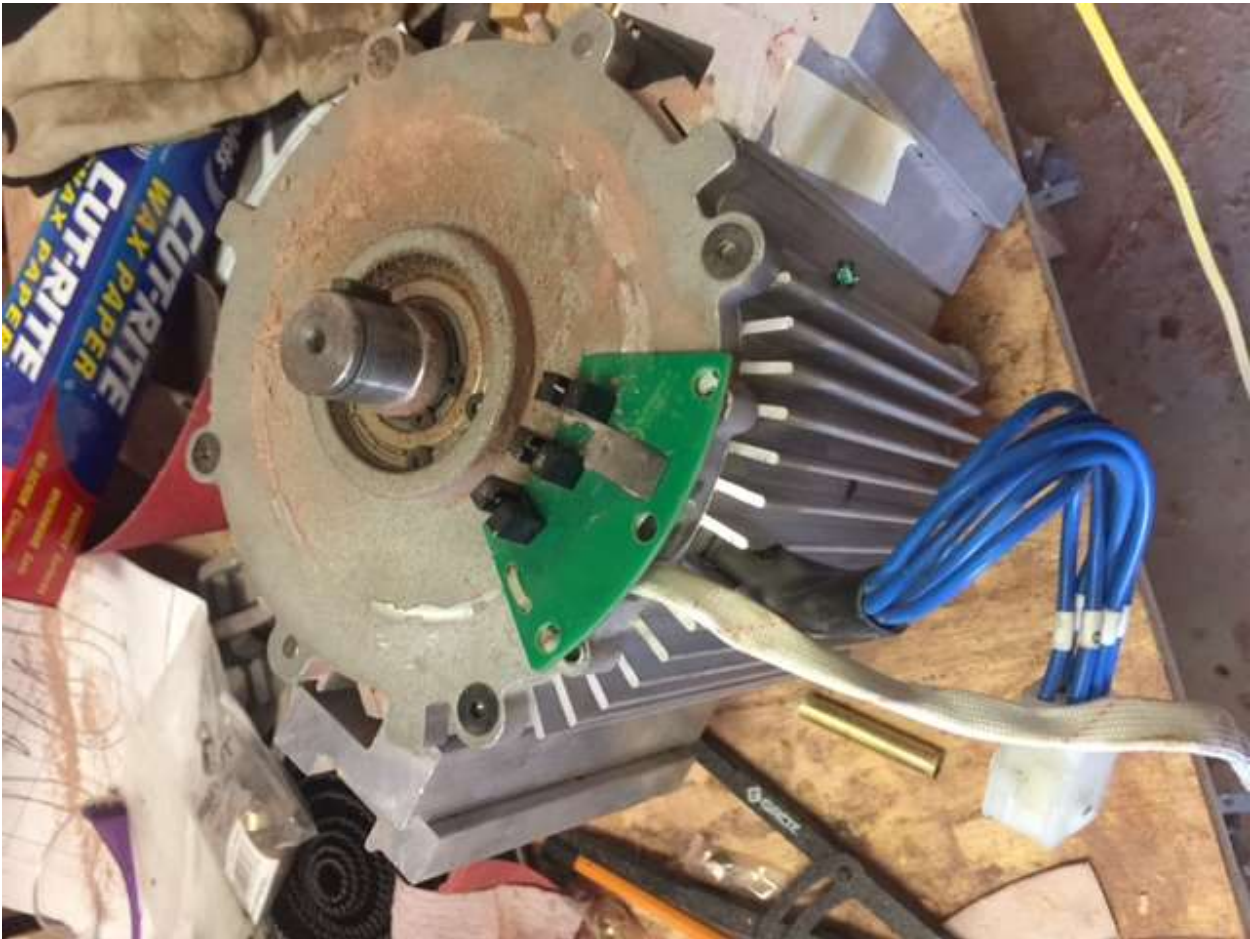
Existing Speed Sensor w screws removed
