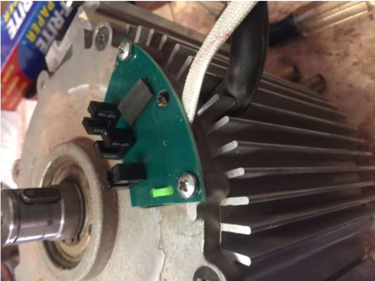
New Speed Sensor Attached to Motor
