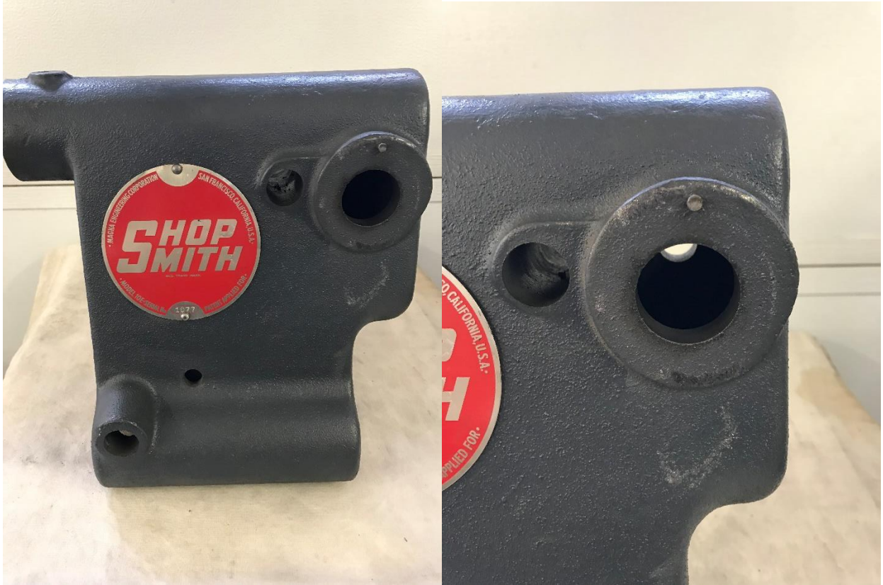
102-1 Headstock for S/N 1077, Note the Pin for the Quill Return Spring Housing and not cast on blocks. The Spring Housing (102-11) is Aluminum. The Pinion Shaft (102-10) is different and does not have flat spots on the end for the Feed Lever Knobs set screws.
