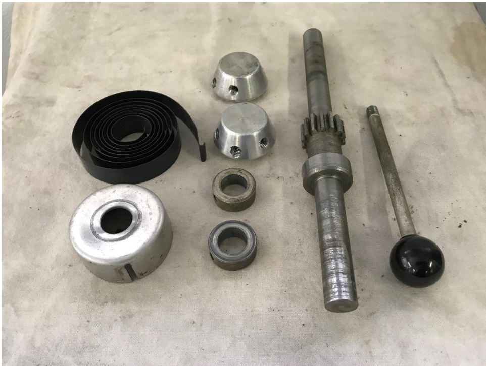
102-1 Headstock for S/N 1077, Note the Pin for the Quill Return Spring Housing and not cast on blocks. The Spring Housing (102-11) is Aluminum. The Pinion Shaft (102-10) is different and does not have flat spots on the end for the Feed Lever Knobs set screws.
