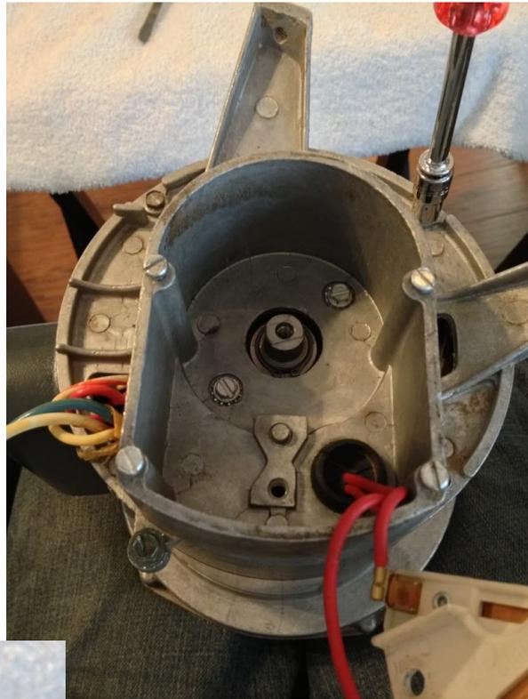
Next, remove the 2 bolts holding the rotor assembly to the rear end cap.
