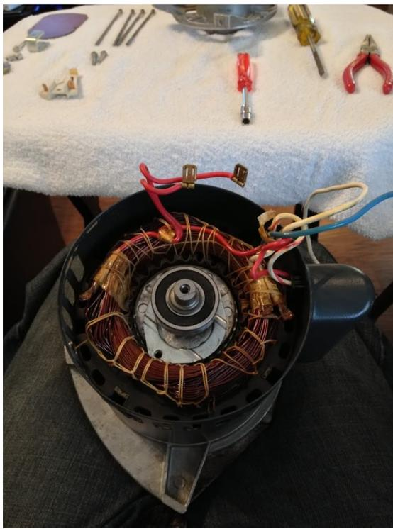
After the rear end cap is removed, gently remove the rotor assembly from the housing.
