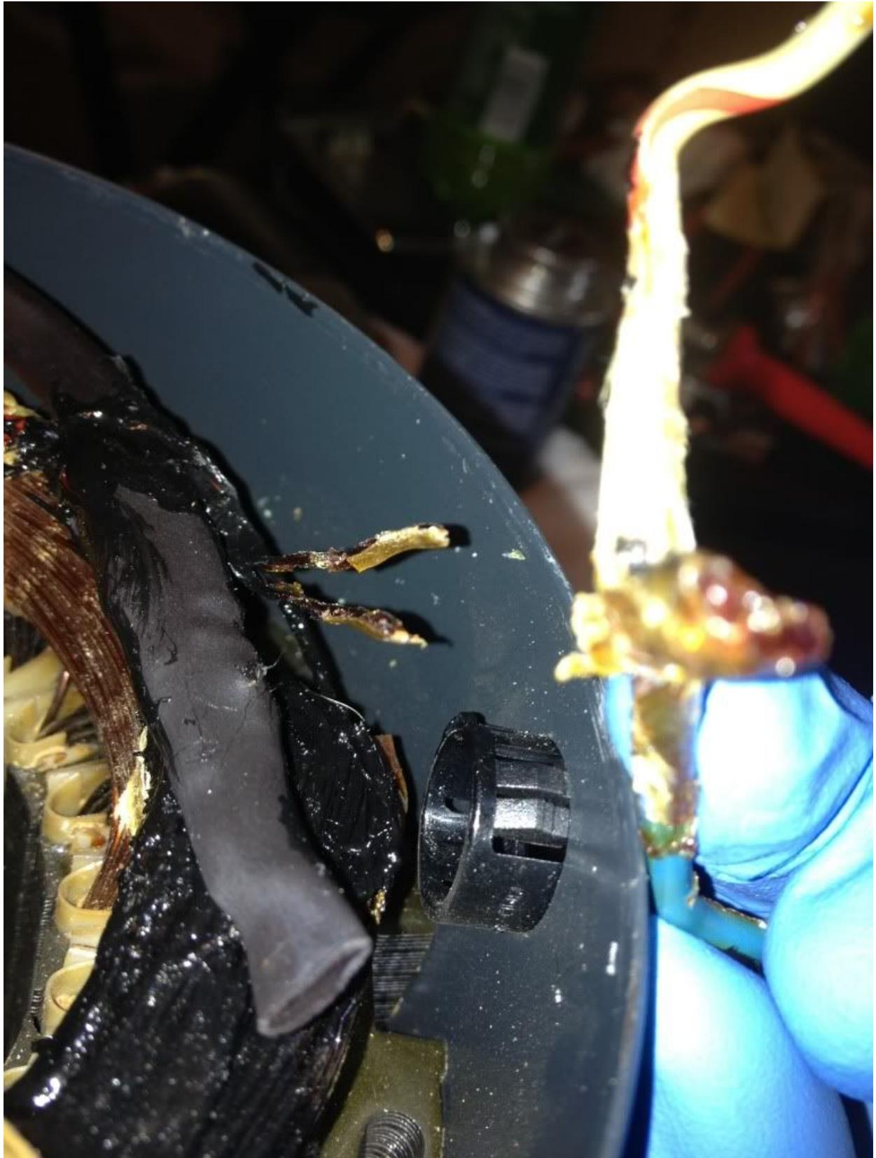
If you are **not** upgrading to 12 gauge wiring, do **not** dissect the splice connecting the [color="Blue"]**blue**[/color] wire and [color="White"]**white**[/color]/[color="Red"]**red**[/color] wire. Instead, cut the [color="White"]**white**[/color]/[color="Red"]**red**[/color] wire off near the splice and insulate it **properly** [color="Red"](*This is a "HOT" wire when in operation*)[/color]. It will not be connected to anything other than the splice it's part of. Skip to the next post.
