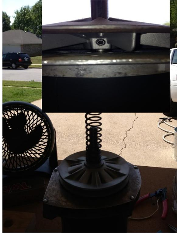
Use a 5/32" allen wrench to remove the set screw at the base of the keyway.
