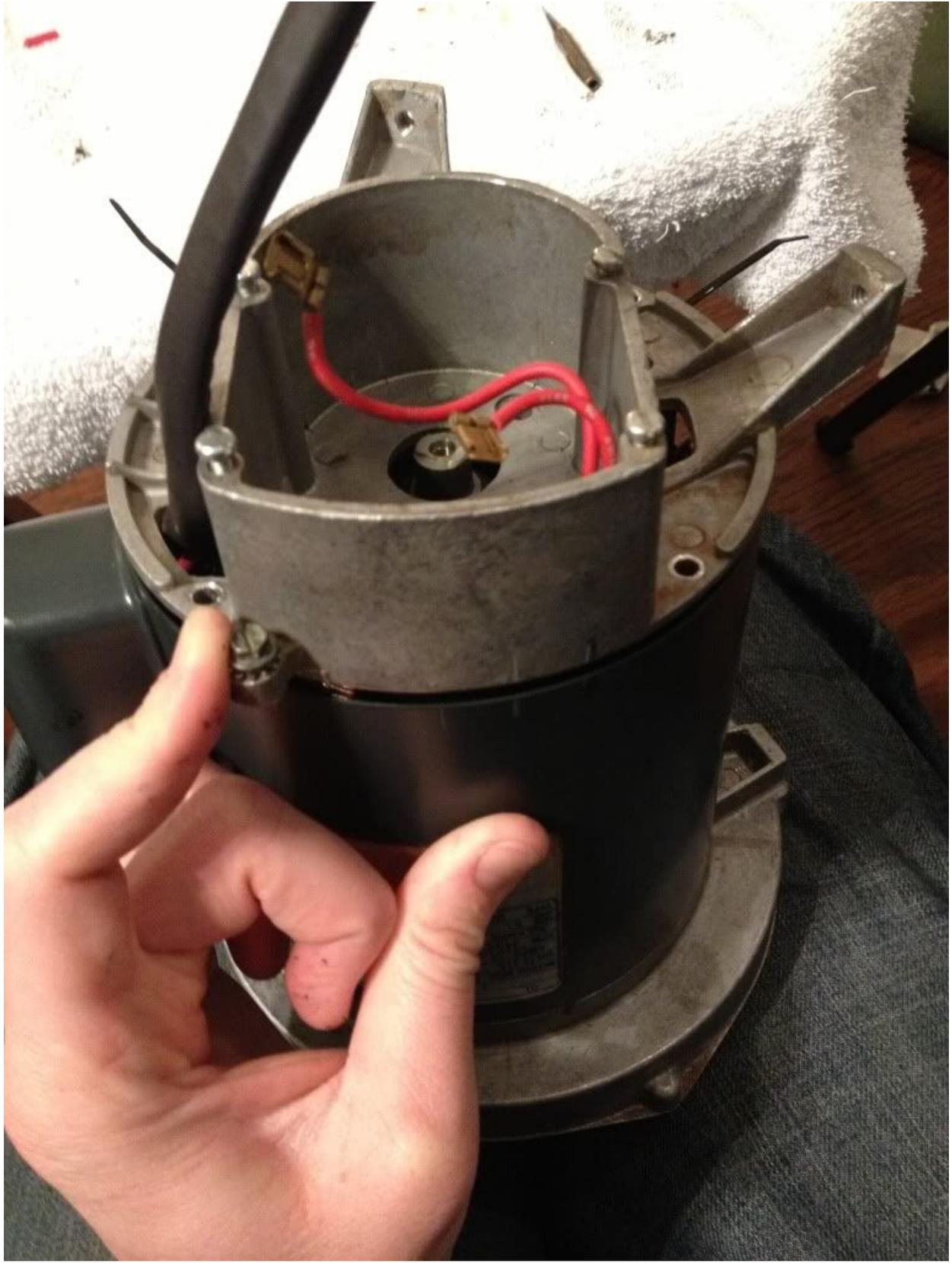
Align the reference marks and seat the rear end cap. The cap will not seat completely until the previously installed zip-ties are removed. Remove the zip-ties and fully seat the end caps and housing. Tighten the rotor assembly screws.
