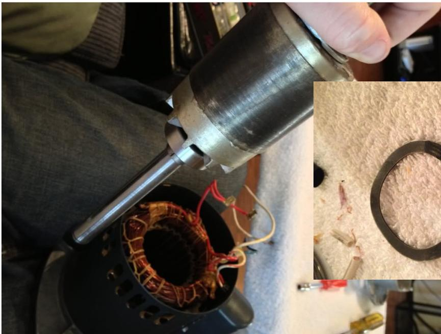
If you are only replacing the bearings and not reversing your motor, re-install the rotor
