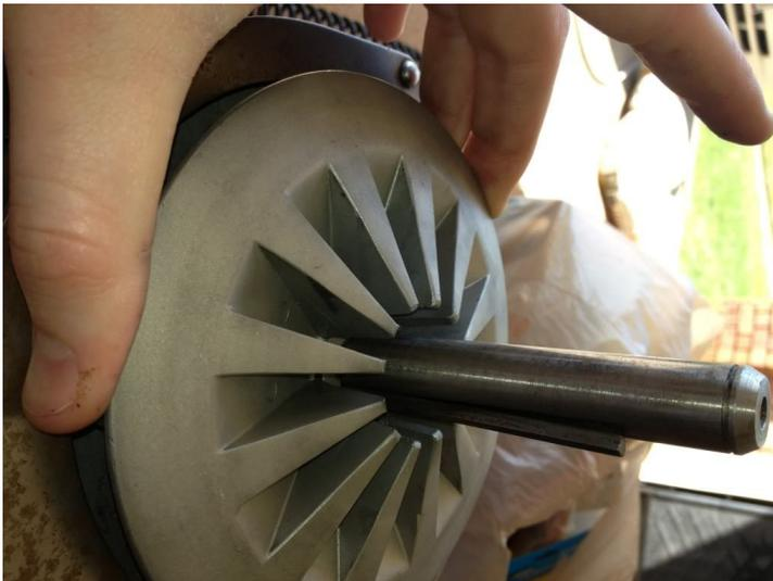
center housing. This is important during re-assembly or the mounting feet will not line up with the motor pan.
