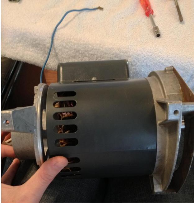
not necessary to move or remove the front-cap. Separate the rear-end cap from the motor housing.
