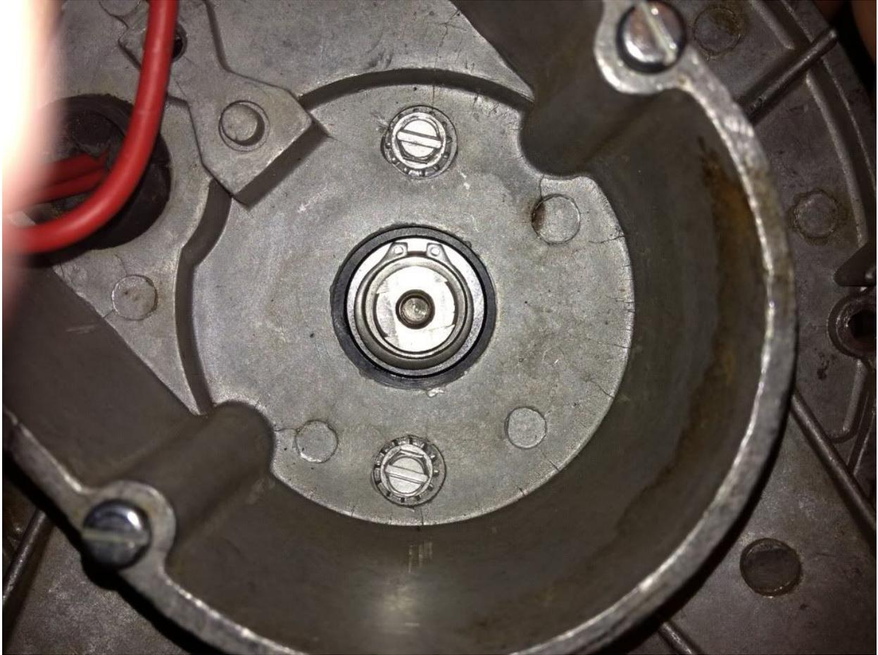
Start and finger tighten the 4 bolts that hold the front and rear end caps together. When installing the bolts, make sure each bolt goes on the outside of the wire bundle to prevent squashing the wires. Two of the bolts will probably require some sort of thin, DULL, reaching tool to manipulate the wire bundle behind the bolt. After all 4 bolts are started, triple check the alignment of the reference marks and tighten the bolts.
