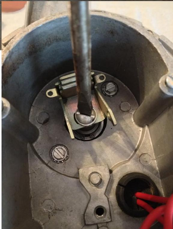
Point the motor towards the floor with the rear facing up. I found holding it between my legs worked very well for these next steps. Use a 1/4" socket to remove the 4 bolts that hold the front and rear end caps to each other.
