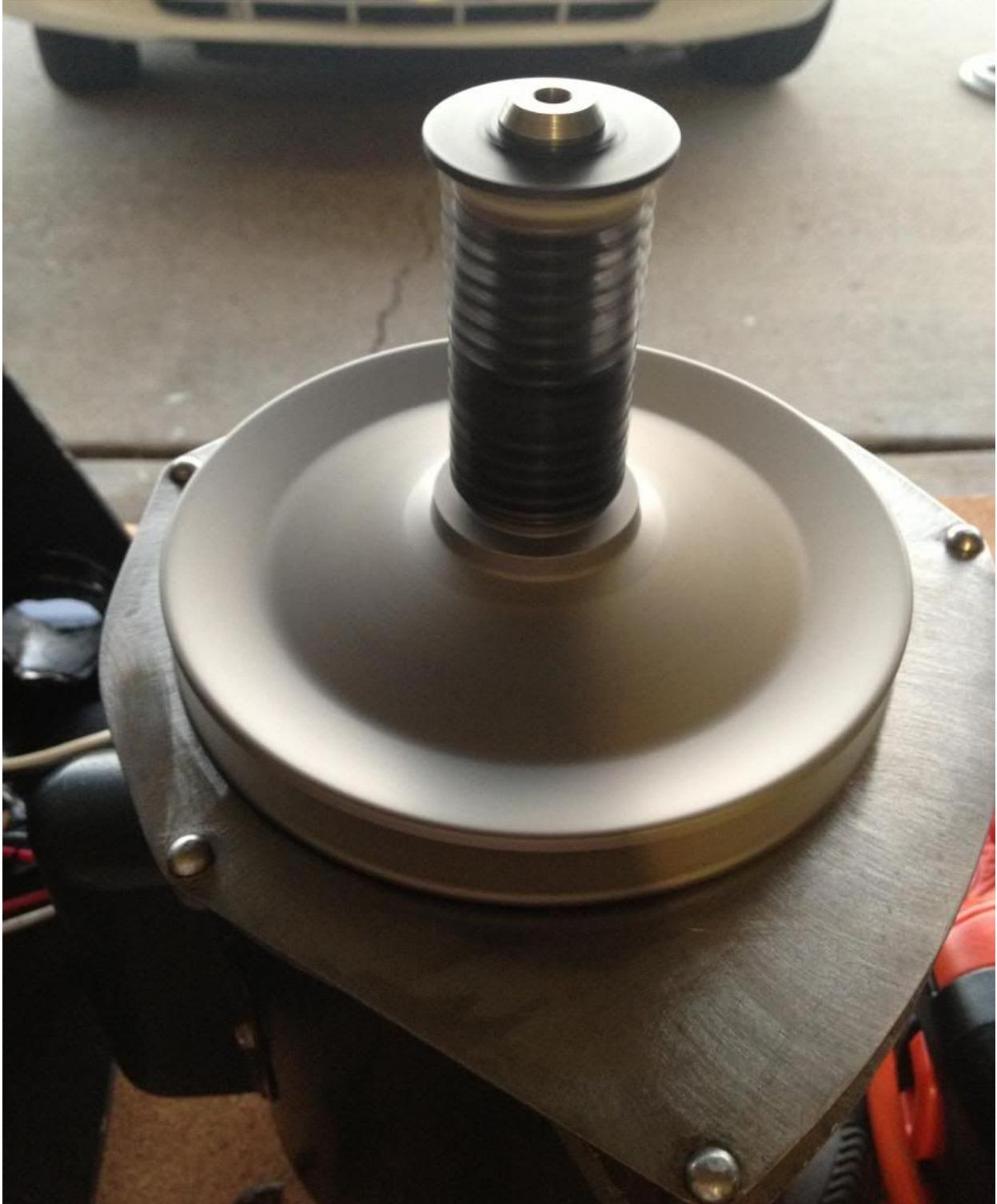
With good bearings (*I used NTN*) and correct installation / tweaking, this motor can be extremely quiet. Below are screen shots of an iPhone app that I used to get decibel readings at 3'. The first is background noise with the motor off, the second is running
