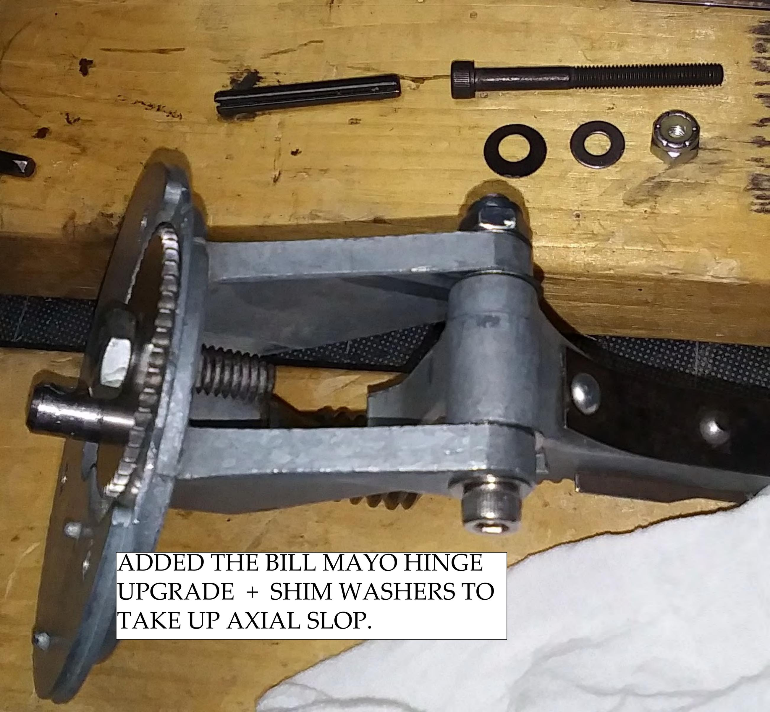
A photograph of a mechanical assembly, likely a hinge, mounted on a wooden workbench. The assembly consists of a grey metal frame with a central cylindrical component. A spring is visible on the left side. Above the assembly, several hardware components are laid out: a long black bolt with a knurled head, a shorter black bolt, two black shim washers, and a silver-colored nut. The workbench is made of light-colored wood, and a piece of white paper is visible in the bottom right corner.
