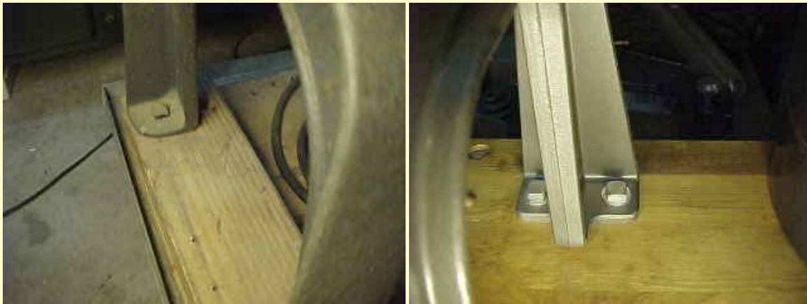
Headrest bolt pattern: one bolt on each side or two on each side
