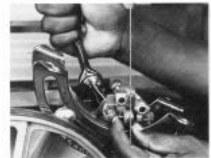
Figure 10. To adjust the lower blade guide roller, loosen the mounting bolt at the back of the bandsaw. Slide the assembly sideways until the roller is centered behind the blade and then tighten the bolt.
